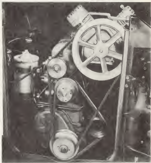
18-47. The truck engine driven refrigeration compressor. (Lehigh Mfg. Co.)
